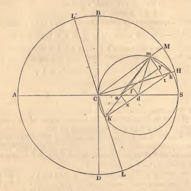
Then the place of high water is where the elevation = maximum, or when  $S \times \cos^2 x + M \times \cos^2 y = maximum$ , and since
